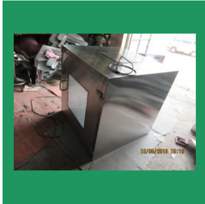
Hatch Pass Box
